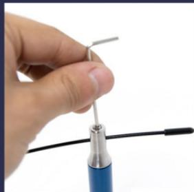
WITH THE HEX KEY PROVIDED, UNSCREW THE TIP OF THE HANDLE TO SET THE DESIRED LENGHT. THEN SCREW TO BLOCK THE ROPE.
